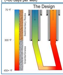
A drilling rig arrives and begins to drill wells with a target depth of 20,000 feet where temperatures are expected to exceed 450 degrees Fahrenheit. If target depths are reached, the two wells will be connected at the base to create a loop.
