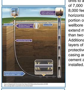
A production rig arrives and drills to a depth of 7.000 to 8,000 feet. The horizontal portion of the wellbore can extend more than two miles. Additional layers of protective steel casing and cement are
