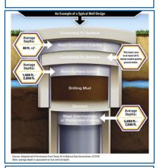
A drilling rig begins the underground construction process by installing steel pipe and cement (surface casing) to protect groundwater. Surface casing is set at least 50' below the aquifer, typically about 1,500+' below the surface.
